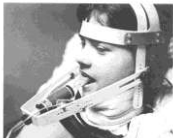
Tongue/Lip Controller Effective wheelchair control for those with little or no head and neck mobility.
